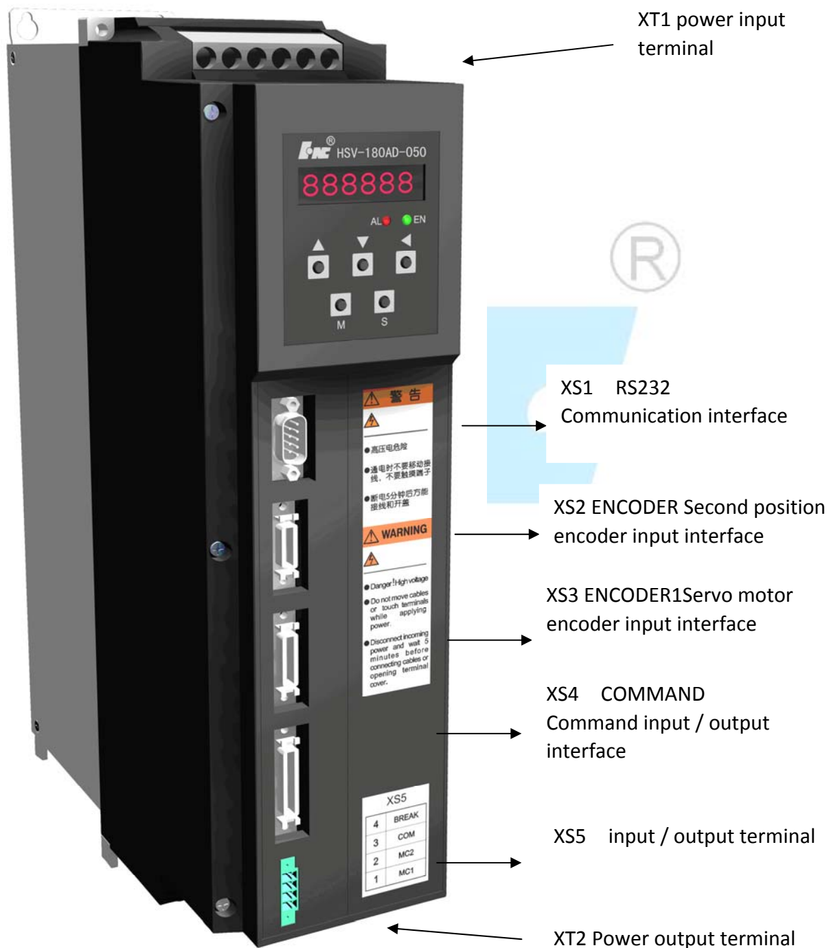
Figure 5-2 Interface configuration of HSV-180AD
