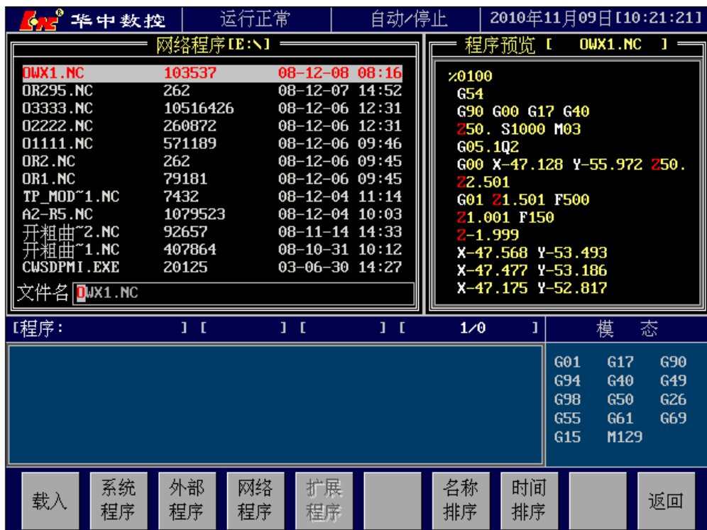
Figure 3-3 Network Program Loading Interface
