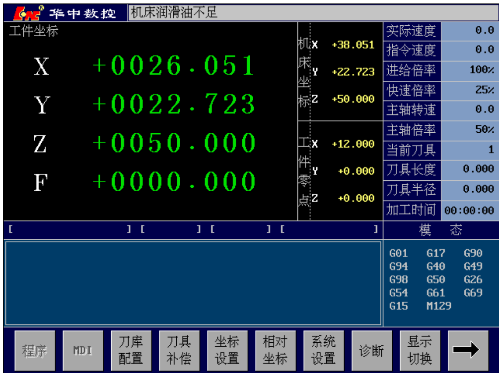
Figure 7-20 System Displays PLC Message
