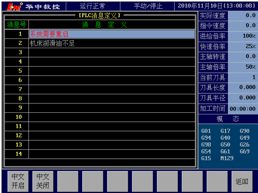
Figure 7-21 PLC Message Definition Interface
