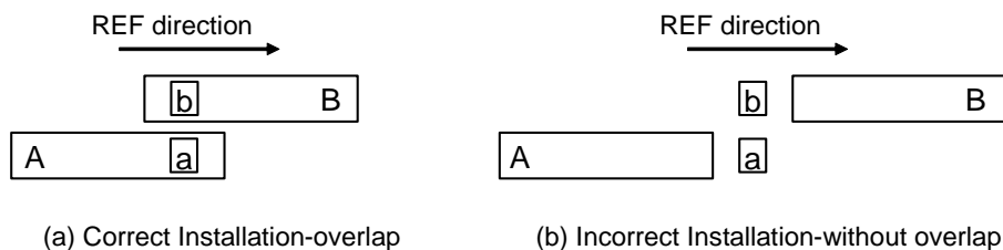
Figure 4-2 Installation of REF switch and over-travel limit switch
