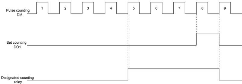
Fig.5-29 Setup counting value&designated counting value schematic diagram
