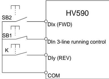
Fig. 5-9 Three-line control mode 2
