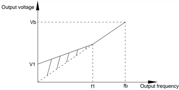
V1:Manual torque boost voltage      Vb:Maximum output voltage
