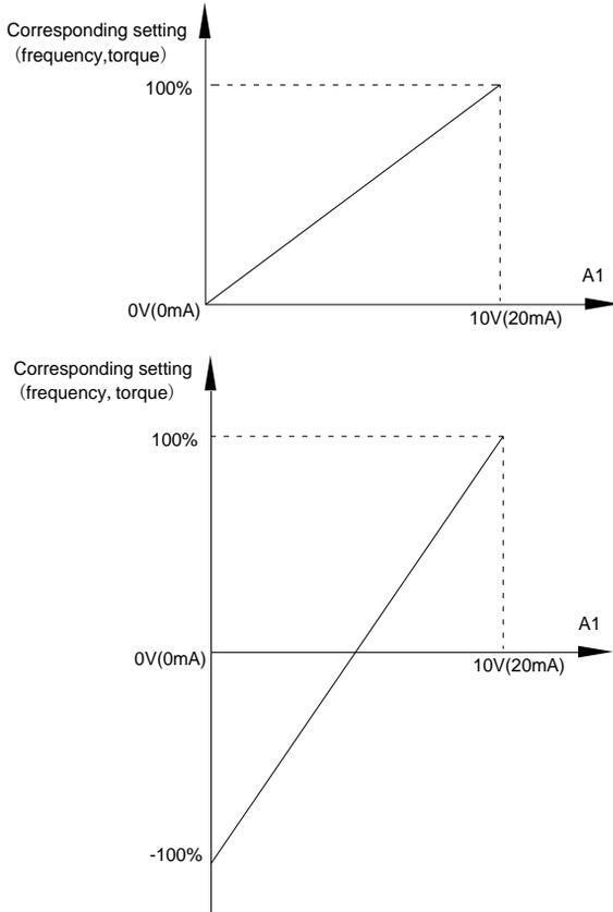
Fig. 5-10 Relationship between analog input and setup value
