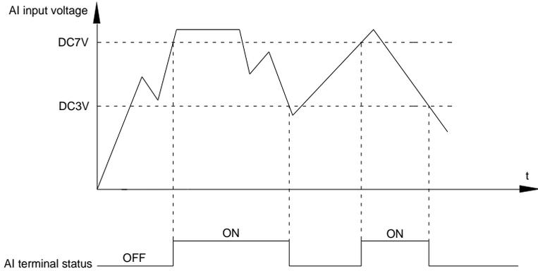
Fig.5-31AI terminal valid state schematic diagram
