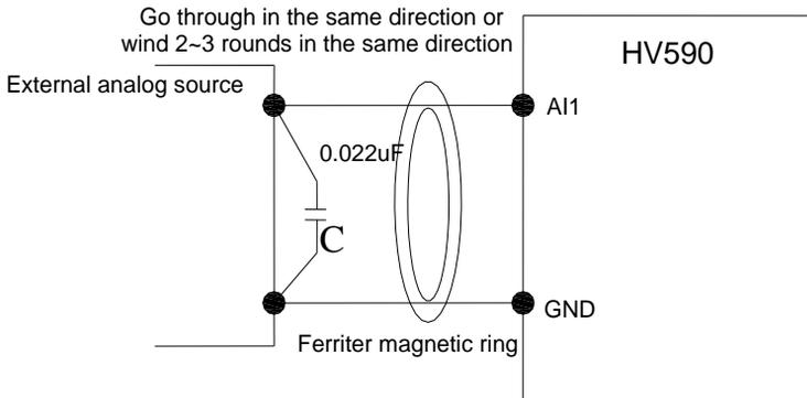
Fig.2-6.2 Analog input terminal processing wiring diagram
