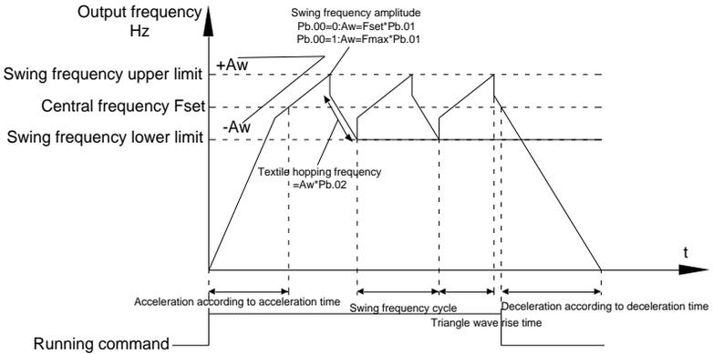
Fig.5-28 Swing frequency schematic diagram
