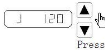
Figure 4-7 Jog trail run without load
